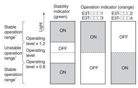
\* If the E3T fs operating level is set to the stable operation range, the E3T will be in most reliable operation without being influenced by temperature change, voltage fluctuation, dust, or setting change. If the operating level cannot be set to the stable operation range, pay attention to environmental changes while operating the E3T.
